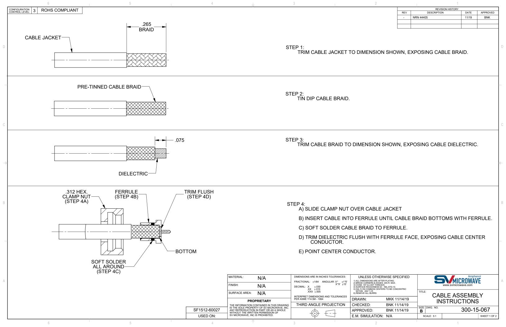
REVISION HISTORY **ROHS COMPLIANT** APPROVED REV DESCRIPTION NRN 44405 BNK STEP 5: INSERT CABLE ASSEMBLY INTO CONNECTOR ASSEMBLY. THREAD CLAMP NUT ON TO CONNECTOR ASSEMBLY THREADS. TORQUE TO 22±2 INCH. LBS. CONNECTOR **ASSEMBLY** CABLE ASSEMBLY MICROWAVE MATERIAL: UNLESS OTHERWISE SPECIFIED DIMENSIONS ARE IN INCHES TOLERANCES: N/A 1) ALL DIMENSIONS ARE AFTER PLATING.
