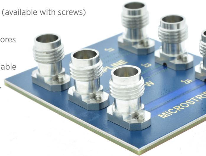
As frequencies increase and board substrates become thinner, the standard solderless PCB compression mount connectors in Figure 1, below, can create undesirable results on thin (< .010") dielectric PCB. The LiteTouch connector, shown in Figure 2, addresses this issue by maintaining a solderless connection while keeping the board material intact.
