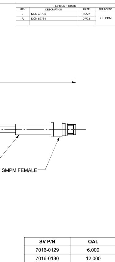
7016-0131 24.000 Amphenol OTHERWISE SPECIFIED MICROWAVE ARE IN INCHES [MILLIMETERS] ARE AFTER PLATING. S & EDGES.005 R. MAX. ST THREADS. HNESS 63₄MIL-STD-10. ON CENTERS TO BE CONCENTRIC & CENTERS TO BE CONCENTRIC 2.4mm MALE TO SMPM TITLE: FEMALE FOR FLEXIBLE .047 CABLE ASSEMBLY KRR 02/25/22 SIZE DWG. NO. 7016-0129-0131 SEE PDM SEE PDM D: SCALE: 4:1 SHEET 1 OF 1
