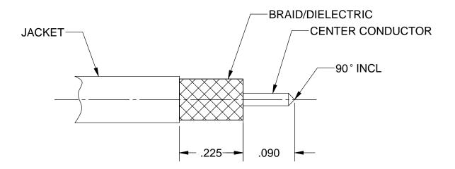
FLUSH-CUT END OF CABLE PRIOR TO REMOVING THE OUTER JACKET. DIP END OF CABLE INTO FLUX AND THEN INTO SOLDER POT, MAINTAINED AT 500°F, TO A DEPTH OF 3/8 INCH FOR 6 SECONDS MAX. SN63 SOLDER IS RECOMMENDED.
