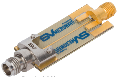
Edge-Lock 2.92mm connector (right) attached to eval board
