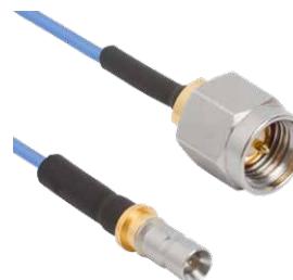
SMPM Male VITA 67.3 to SMA Male Cable Assembly for Ø.047" Cable SV PN: 7032-7841 (12")
