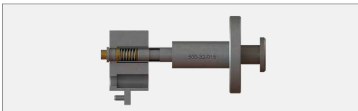
Figure 9.6 Contact Removed. Uses Tool PN 500-32-015.
