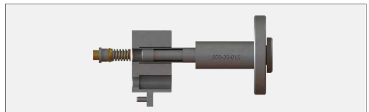
Figure 9.7 Contact Removed from Block
