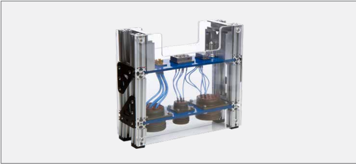
Figure 4 VITA Sample Chassis with 67 RF Modules Terminated to D38999 Circular Connectors with Coaxial Contacts
