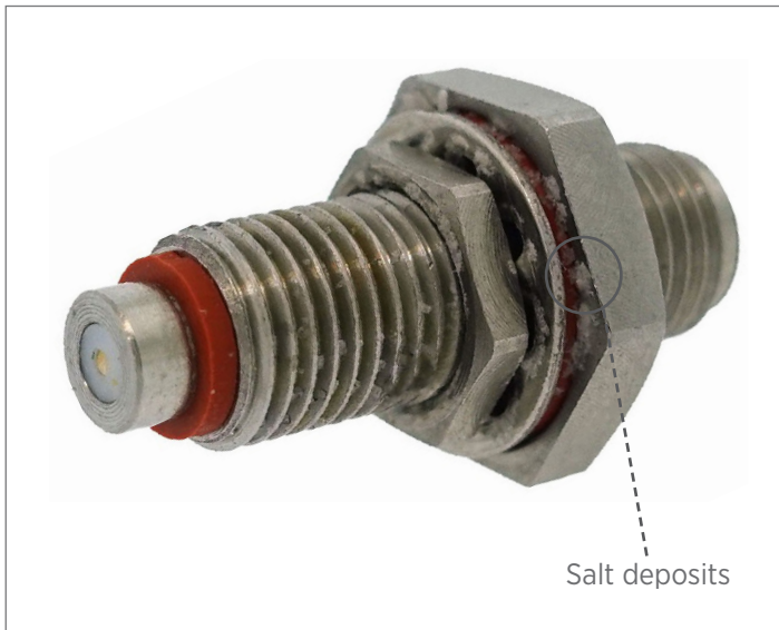
Figure 1: LTI female to SMA female bulkhead adapter with salt.
