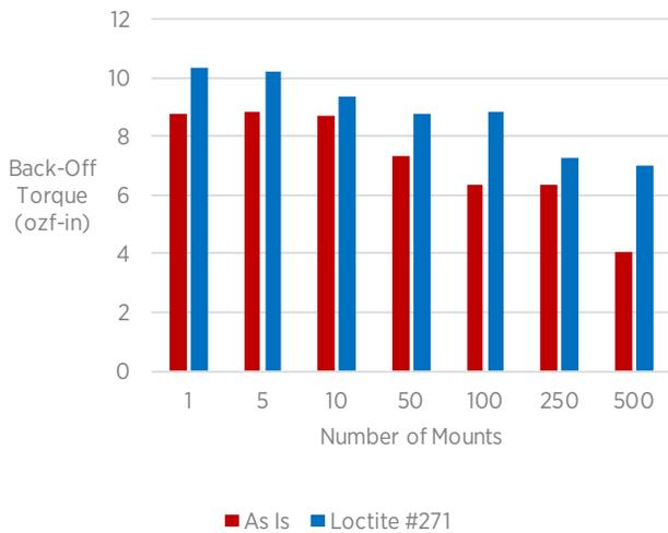
For this test, mounting screws were fully tightened then removed to simulate the effects of removing and placing connectors in multiple locations.
