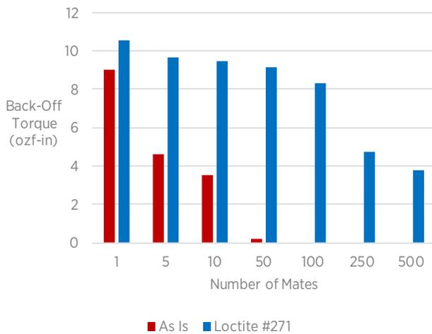
For this test, the mounting screws were fully torqued then a connector was mated and unmated. This was meant to simulate a high mating cycle environment.
